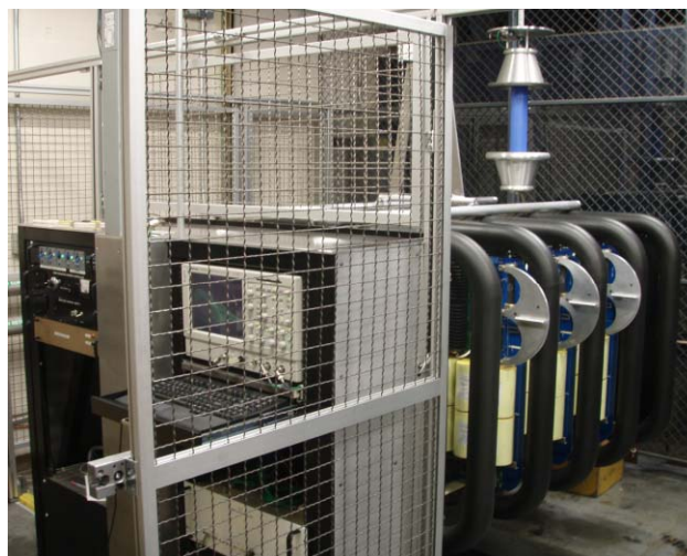
Figure 1. The ILC Marx Modulator in Testing Area.
