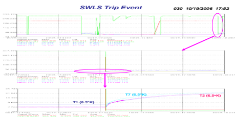
(a) Control system 10 sec logger data shown that the SWLS trip happened.
