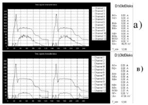
Figure 3: Oscillograms for the closed mode of magnetron gun operation. a) in the rising magnetic field; b) in the falling magnetic field.
