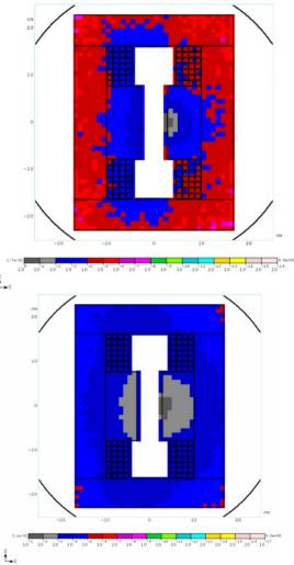
**Figure 4:** Cross sectional energy distribution, showing the energy deposited in the coil packs at 500 MeV (top) and 5 GeV (bottom) incident energy.
