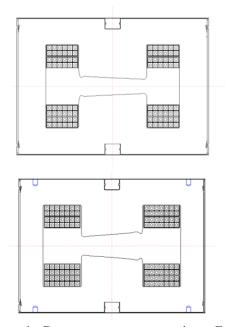
Figure 1: Booster magnet cross sections. Each magnet is approximately 13" high by 18" wide.
