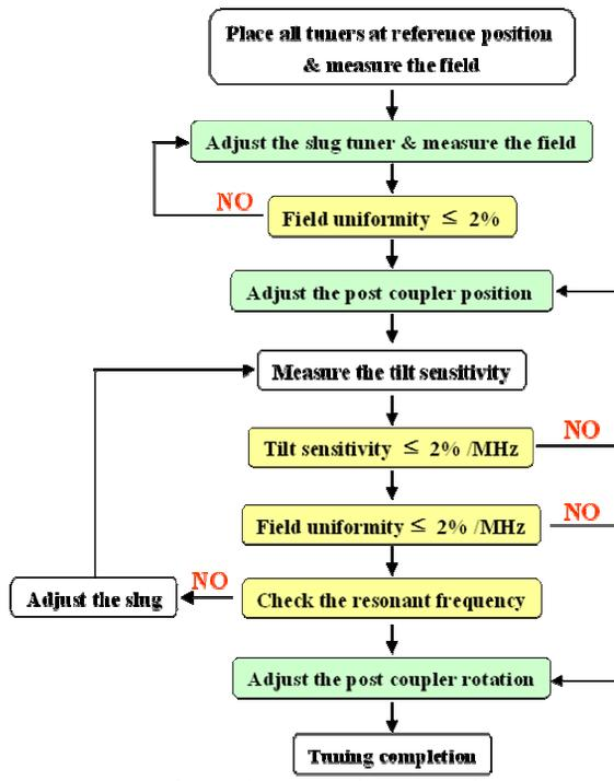
Figure 4: DTL tuning procedure
