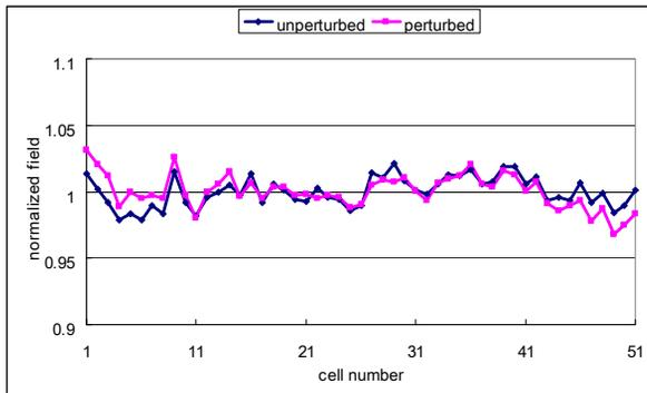
Figure 7b: Field profile after post coupler adjustment
