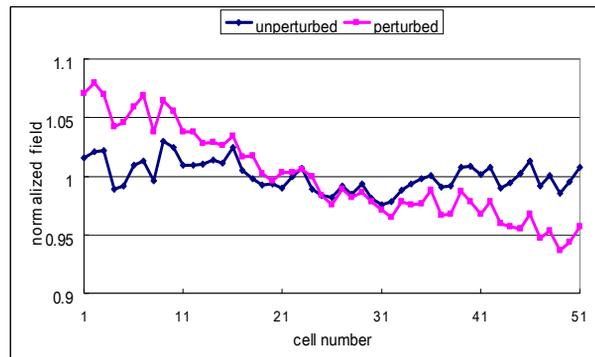
Figure 7a: Field profile before post coupler adjustment
