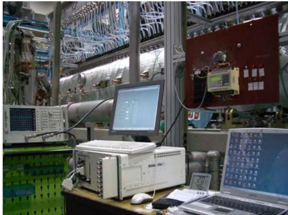
Figure 3: Tuning Setup for DTL tank 1
