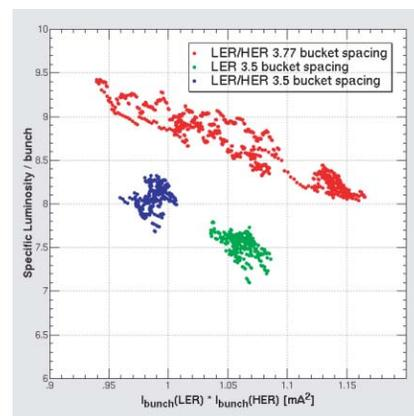
Figure 3: An old experiment showing lower specific luminosity with shorter bunch spacing. This data was taken on June 19 2004.
