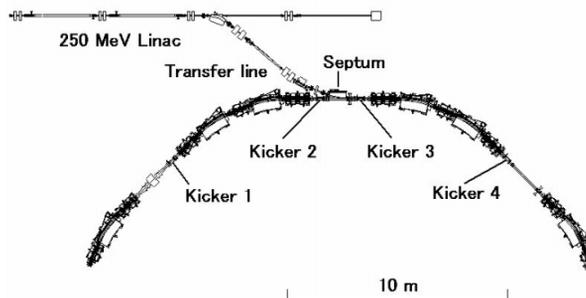
Figure 1: Injection area of SAGA Light Source
