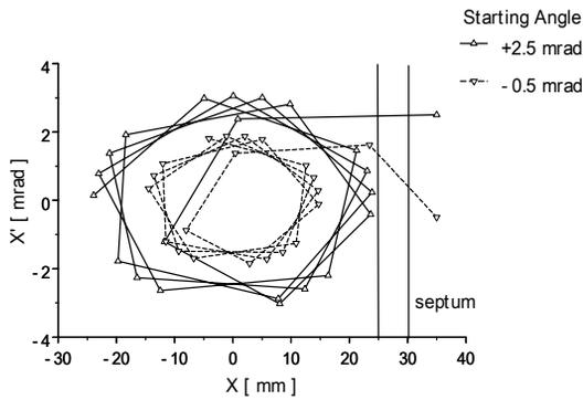
Figure 6: The angle acceptance with the nominal bump
