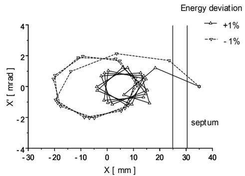
Figure 9: The energy acceptance for the nominal injection.
