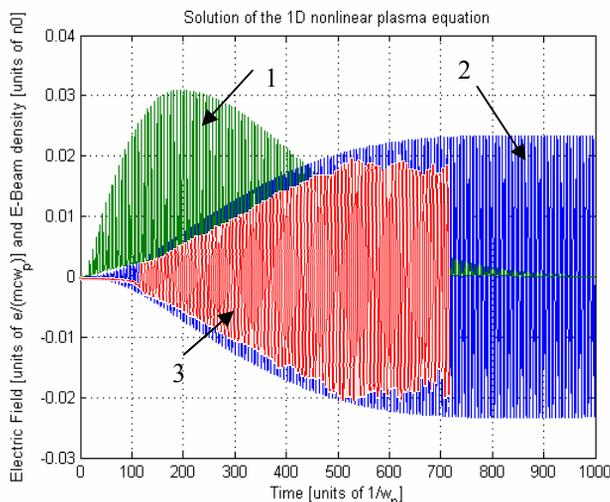
Figure 1: The electron beam density  $\times 100$  (1), the theoretical wakefield (2) and simulated wakefield (3) after 1mm of propagation in the plasma.
