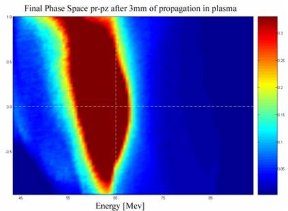
Figure 2: The final phase space of the beam after the exit of the 3mm long plasma. The density is in units of the plasma density, the horizontal axis in MeV and the vertical in units of mc.
