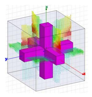
Figure 2: Cell of wire lattice, square cross section of width w=0.1 cm, period d=0.58 cm. The plasmon mode at 20.85 GHz is calculated for the phase advance of 60 deg. in the *x* direction, and 0 in the *y* and *z* directions. **E**-vectors are plotted in the *x*, *y*, *z* planes. Amplitude is ranged from 1 (red) to 0.1 (blue).
