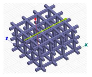
Figure 1: Metallic photonic crystal built as a cubic lattice of intersecting square wires. The green arrow represents an electron beam passing above the lattice.
