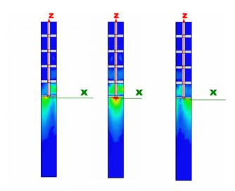
Figure 4: Stack of cubic cells and field intensity. The surface mode localized at the interface. The period d=0.58 cm, wire width w=0.1 cm. The surface mode is calculated at frequency of 20.45 GHz for the phase advance of 150 deg. in the *x* direction. The snapshots at  $\omega t=-60$  deg., 0, and 60 deg., respectively, show opposite directions of wave propagation in vacuum and the lattice. The field amplitude is ranged from 1 (red) to 0.1 (blue).
