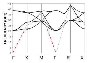
Figure 3: Brillouin diagram for the metallic wire lattice. The period d=0.58 cm, wire width w=0.1 cm. The free space dispersion lines are shown as blue dashed lines. The lower frequency mode is a plasmon mode. Red dashed line - the dispersion of the surface mode.
