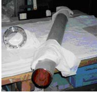
Figure 3: A test stainless-steel chamber coated with copper (“Cu coated chamber”).
