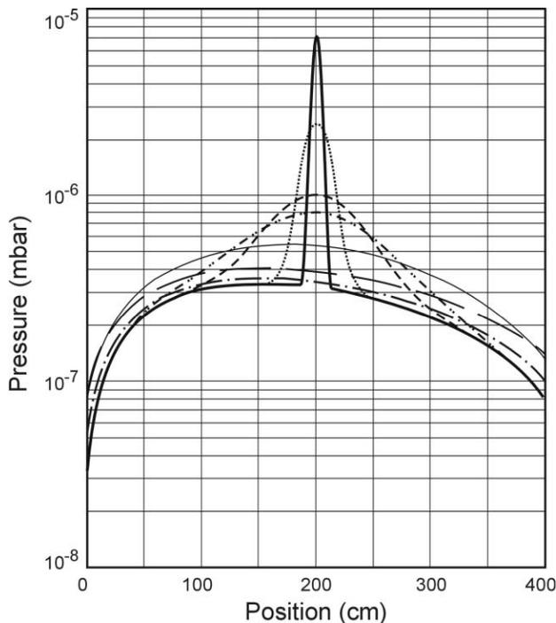
Figure 2: Pressure field along the axis of the conic tube: at  $t = 10^{-4}$  s (thick solid line);  $t = 10^{-3}$  s (dotted line);  $t = 10^{-2}$  s (dashed line);  $t = 2 \times 10^{-2}$  s (two-dot-dashed line);  $t = 10^{-1}$  s (thin solid line);  $t = 10^0$  s (long-dashed line);  $t = 10^1$  s (dot-dashed line).
