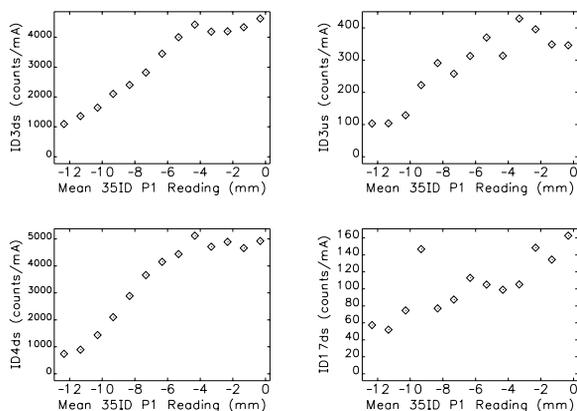
Figure 5: Measured loss rates at several IDs as a function of bump position in ID35.
