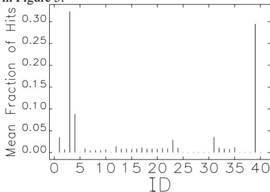
Figure 3: Simulated distribution of losses in the APS due to Touschek scattering, with the horizontal scraper in its nominal position.
