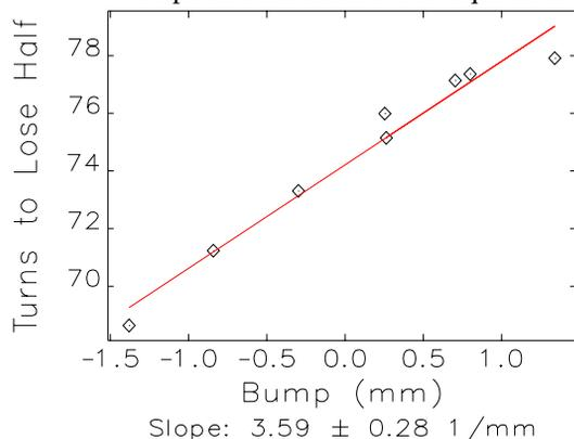
Figure 1: Measured number of turns required for half the beam to be lost following gating off of the rf drive, as a function of bump height in ID3 and ID4.
