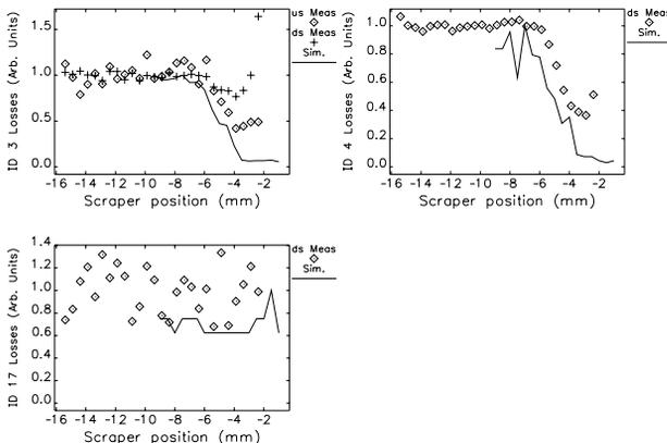
Figure 4: Simulated and measured loss rates at several IDs as a function of scraper position.
