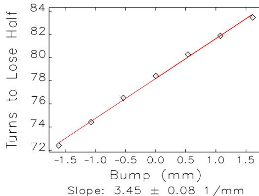
Figure 2: Simulated number of turns required for half the beam to be lost following gating off of the rf drive, as a function of bump height in ID3 and ID4.
