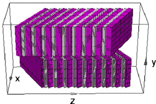
Figure 4: Schematic drawing of the tilted configuration. Thick blocks and thin blocks represent VP poles and magnets, respectively.
