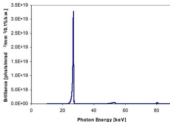
Figure 6: Brilliance from a 15-mm-period tilted hybrid staggered undulator. The calculation was done by using XOP [9].
