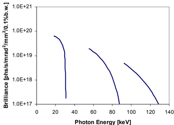
Figure 3: Tuning curves of peak brilliance from a 15-mm-period hybrid staggered undulator. Electron energy: 7 GeV, emittance: 2.5 nmmrad, coupling: 1%.
