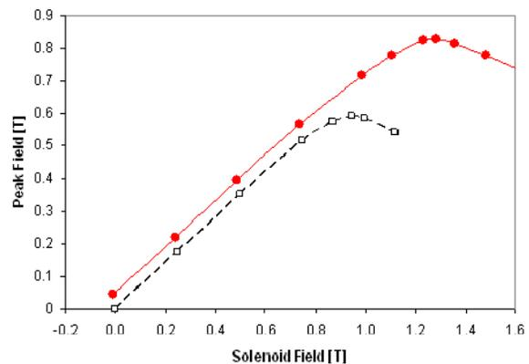
Figure 2: Vertical peak field variation as a function of the longitudinal solenoid field. The solid curve with solid circles represents the peak field variation of the hybrid staggered undulator, and the broken curve with open squares represents the field variation of a conventional staggered undulator.
