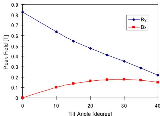
Figure 5: Horizontal-field  $B_x$  (square) and vertical-field  $B_y$  (diamond) variation as a function of tilting angle at a gap of 6 mm. The period length was kept constant at 15 mm. Constant solenoid field (1.28 T) was assumed.
