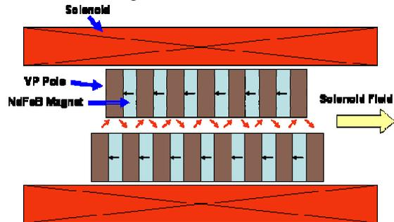
Figure 1: Schematic of a hybrid staggered undulator.
