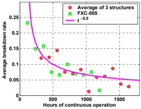
Figure 2: Breakdown rate as a function of time.
