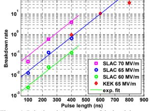
Figure 4: Pulse length dependence of the breakdown rate.
