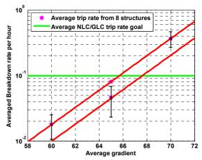
Figure 3: Average breakdown rate as a function of accelerating gradient.
