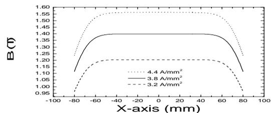
Figure 2: The distribution of vertical field in the medium plane with various current excitation.
