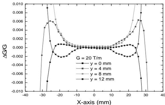
Figure 4: The homogeneous gradient field as a function of horizontal position at four vertical positions in the good gradient region.
