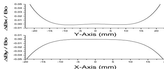
Figure 7: The calculated field distribution of the horizontal and vertical steering coils in the sextupole magnet.
