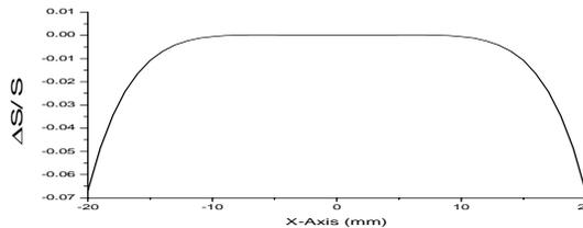
Figure 5: Predicted uniformity of the sextupole field strength of 640 T/m<sup>2</sup> in the transverse direction.
