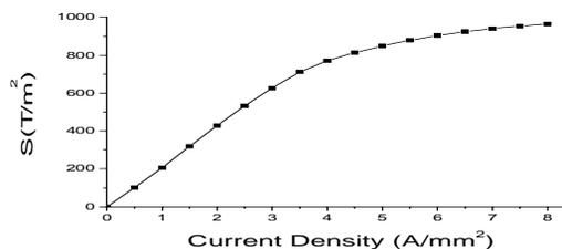
Figure 6: Calculated sextupole field strength as a function of excitation currents.
