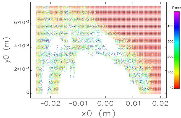
Figure 1: APS dynamic aperture (without physical apertures). The color indicates the number of turns survived before loss.
