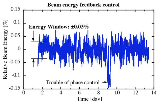
Figure 3: Beam energies stabilized by feedback controls.
