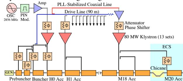
Figure 1: RF system of SPring-8 linac.
