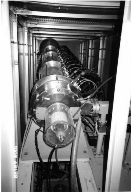
Figure 1: View of structure of the 9MeV TW linac from the electron gun side.
