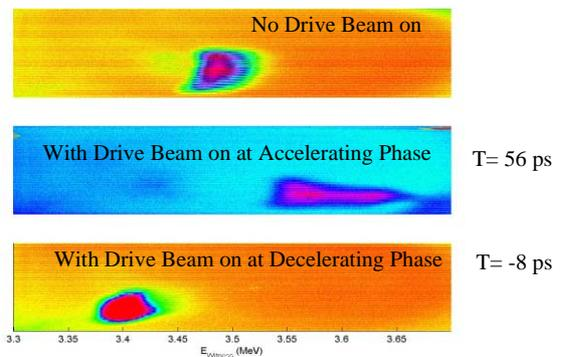
Figure 3 Measured energy change of the witness beam. The top is with drive beam off and middle is with drive beam on and with a cceleration phase of beam delay at 56 ps. The bottom shows the deceleration.
