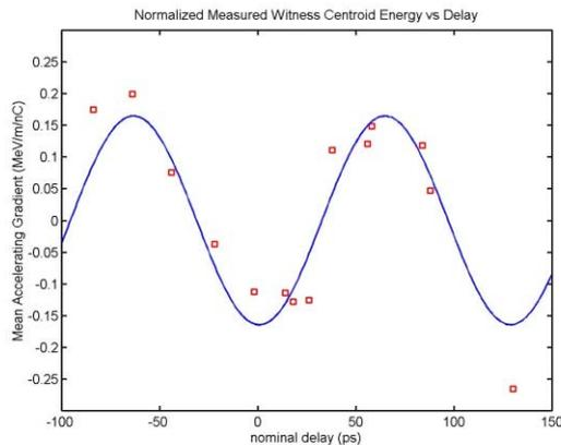
Figure 4 Measured witness beam centroid energy change vs delay.
