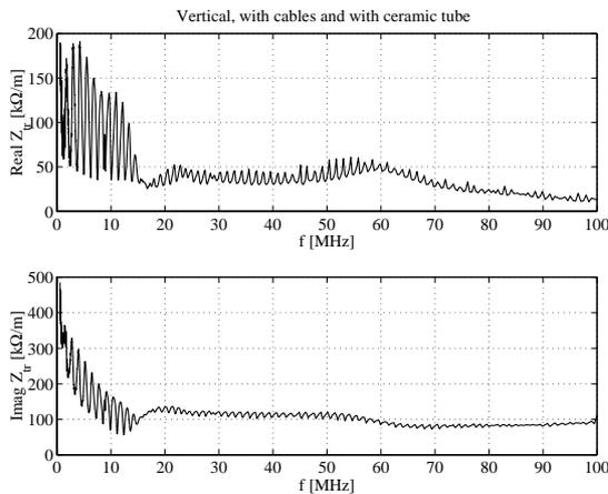
Fig.1. Vertical transverse impedance of TW injection kicker.
