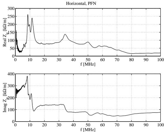
Fig.3. Horizontal transverse impedance of abort kicker with the PFN pulser connected.
