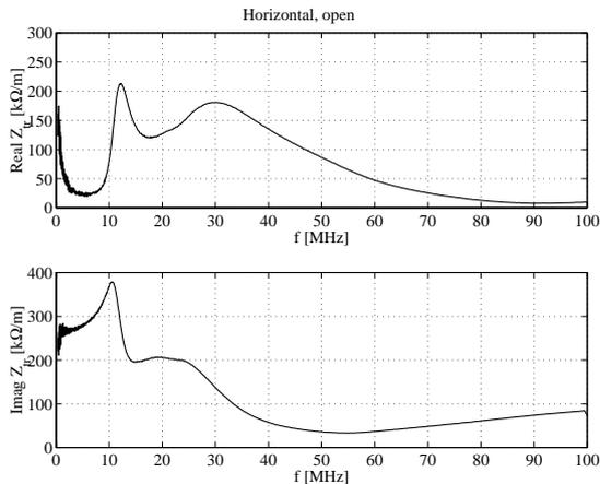
Fig. 4. Horizontal transverse impedance of abort kicker without external load.
