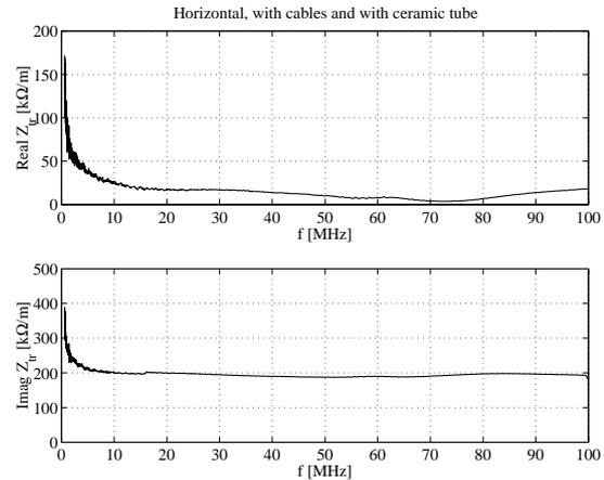
Fig. 2. Horizontal transverse impedance of the TW injection kicker
