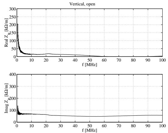
Fig.5. Vertical coupling impedance of abort kicker without external load.
