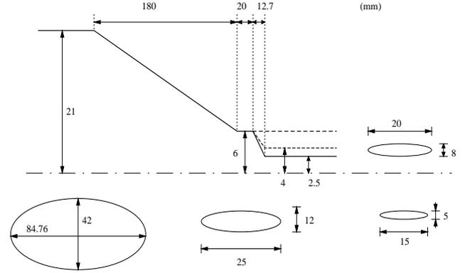
Figure 1: Schematic drawing showing transition from regular to ID chamber.
