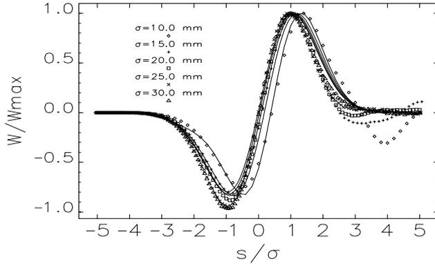
Figure 2: Wake potentials from MAFIA simulation.
