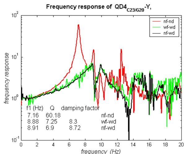
Figure 2: Lateral frequency response functions of the quadrupole QD4 in cell 23 for the frequency range of 0-20Hz, with (wd) and without (nd) damping links in the cases of cooling water flow on (wf) and off (nf).
