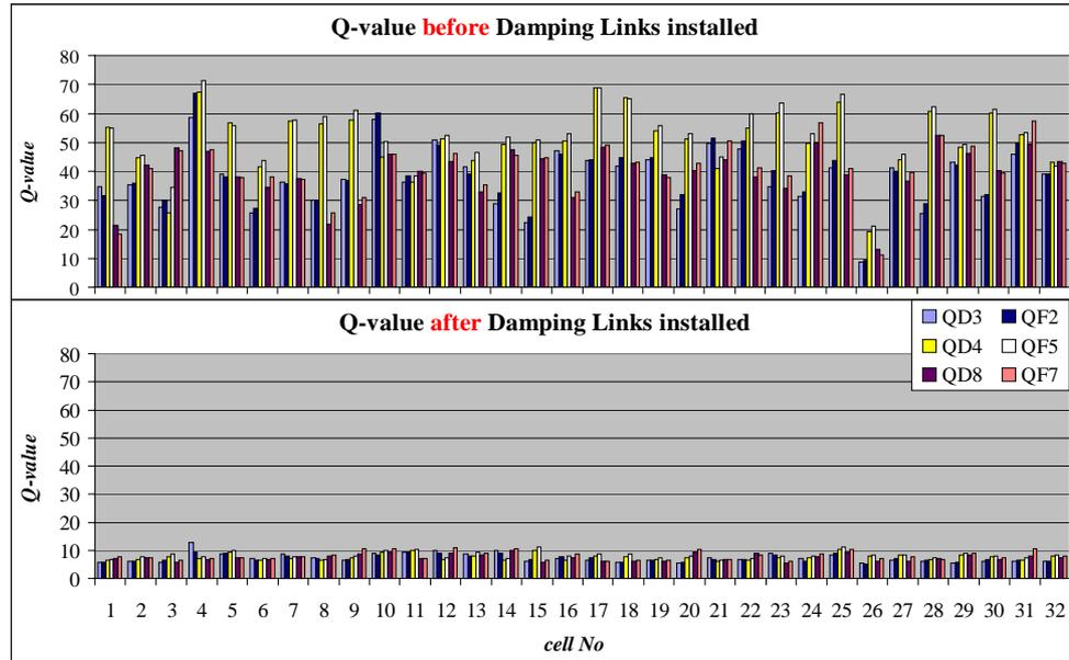
Figure 2: Q-value of quadrupoles before and after the installation of the damping links in the storage ring.
