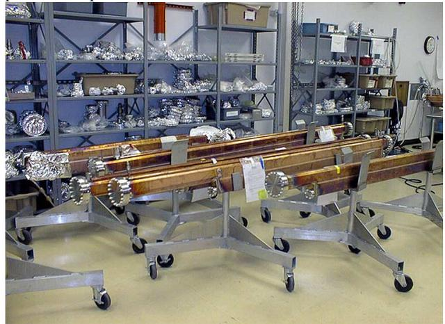
Figure 1: Several of the 60 IR2 Vacuum Chambers during assembly in the SLAC cleanroom.
