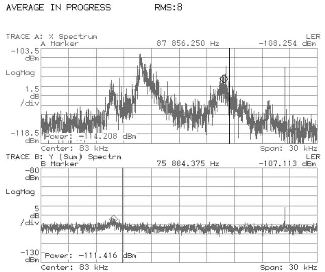
Fig. 1: LER tune spectrum with colliding beams: 1550 mA (LER) on 850 mA (HER). The spectrum shows a lot of structure, which make it hard to use it as a feedback.
