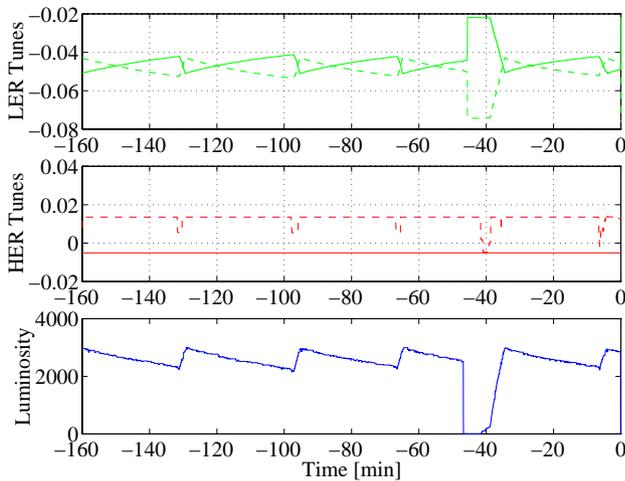
Fig. 3: LER and HER tunes as a function of time. The  $x$  (solid) and  $y$  (dashed) tunes are calculated backwards from the tune quad setting, including the part from the feed-forward and the operator tweaks.
