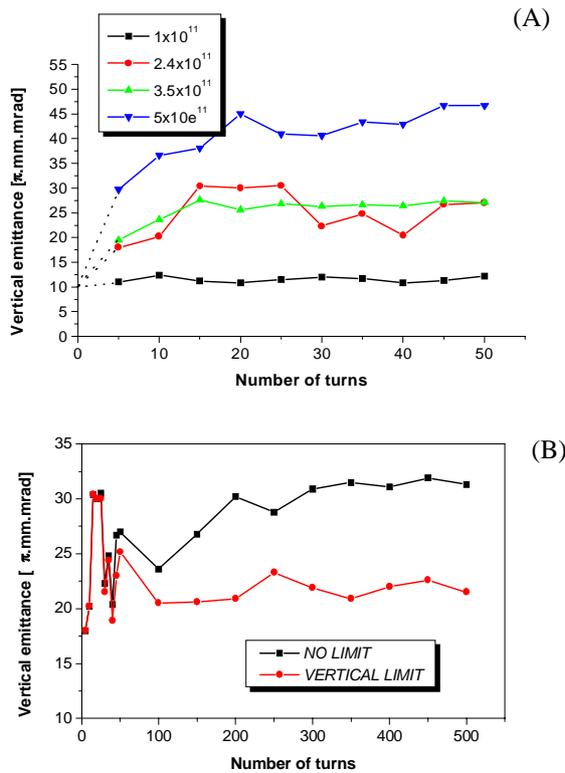
Figure 1: Changing of the vertical emittance caused by the fourth integer resonance exited by the beam.
