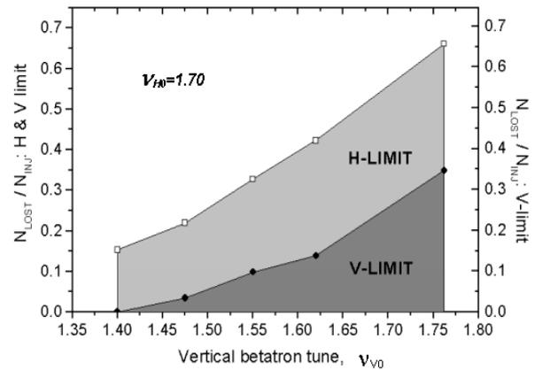
Figure 4: Changing of the particle losses in the horizontal and vertical planes during the injection process for different ‘bare’ working point positions.
