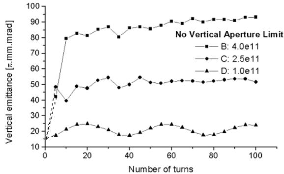
Figure 3: Changing of the vertical beam emittance of the beam at the beginning of the capture process in the case of the ‘bare’ working point near the coupling resonance without vertical limitation of the camber.
