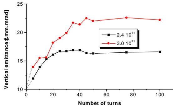
Figure 2: Changing of the vertical beam emittance for different beam intensities in the case of the corrected ‘bare’ working point position.
