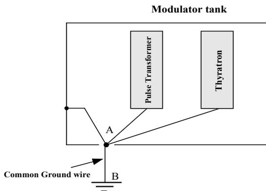
Figure 1: Sketch-map of the common ground wire.
