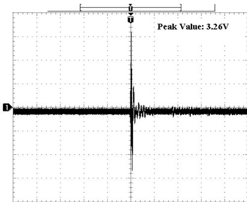
Figure 6: Noise curve after adopting shielding measure to the cable.
