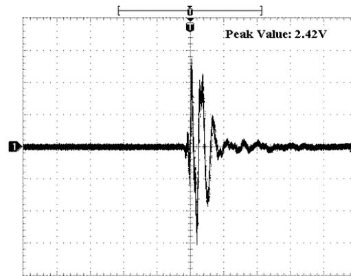
Figure 3: Noise voltages after adopting shielding measure to the common ground wire.
