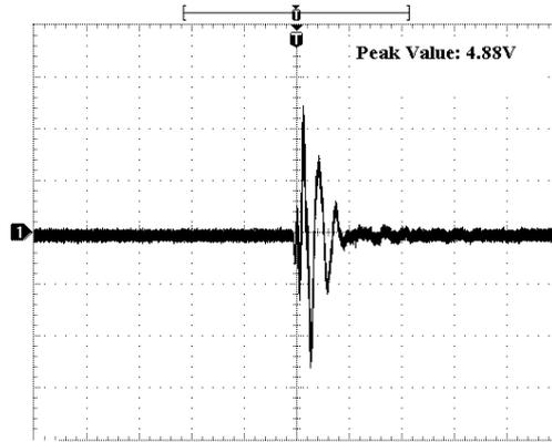
Figure 2: Noise voltages before adopting shielding measure to the common ground wire.
