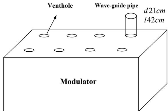
Figure 8: Sketch-map of cut-off wave-guide venthole of modulator.
