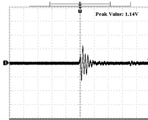
Figure 10: Noise curve after adopting cut-off wave-guide.
