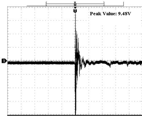
Figure 5: Noise curve before adopting shielding measure to the cable.
