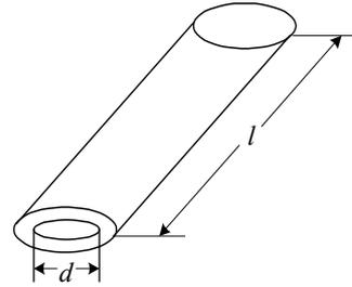
Figure 7: Structure of rotundity wave-guide pipe.
