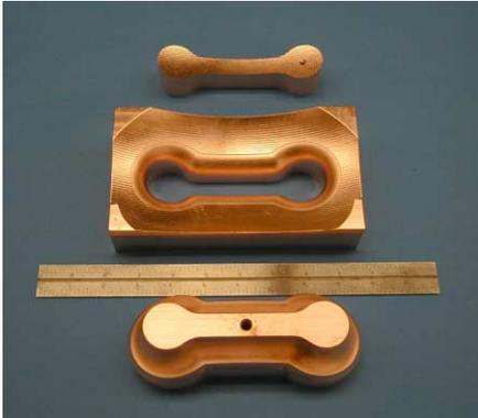
Figure 9. Plunge EDM sample with tellurium copper electrode (bottom) and wire burnout (top).
