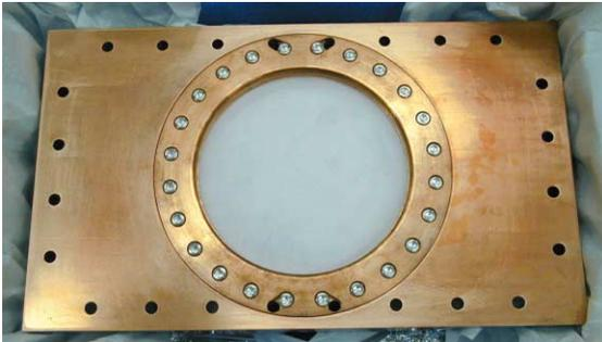
Figure 10. Finished window in waveguide flange.
