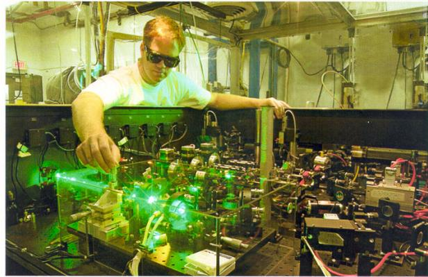
Figure 2. Author making a Ti-sapphire laser adjustment. The Ti-sapphire and diode lasers at Jefferson Lab are remotely controlled and operate for weeks unattended within the injector tunnel.
