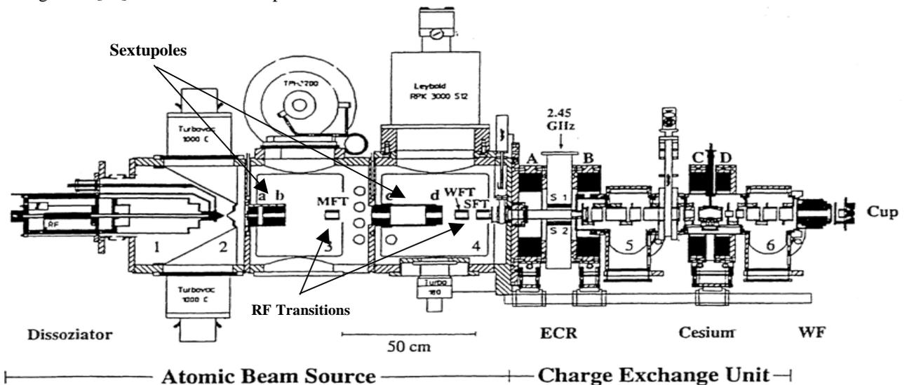
Figure 2: A schematic drawing of the Munich atomic beam polarized ion source, showing the principal components needed to produce a polarized H<sup>-</sup> or D<sup>-</sup> beam.
