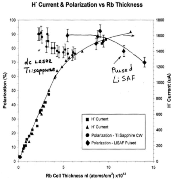
Figure 3: The  $H^-$  beam polarization and output current obtained with the RHIC OPPIS source when installed for early tests at TRIUMF. This shows that significantly increased polarization is obtained with the pulsed  $Cr^{3+}:LiSrAlF_4$  laser, especially at higher Rb vapor thickness in the charge-exchange region.
