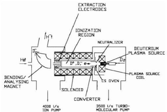
Figure 4: Schematic diagram of the resonant charge-exchange plasma ionizer developed at INR-Moscow.
