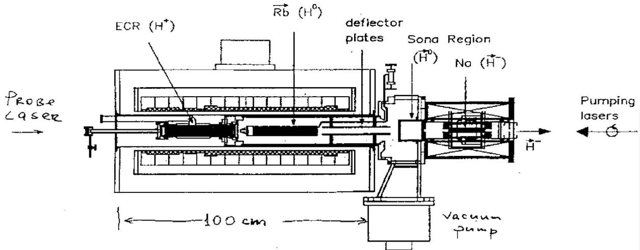
Figure 1: A schematic drawing of the OPPIS-type source installed at TRIUMF, showing the principal components required to produce a polarized H beam.
