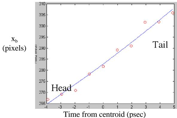
Figure 2: Analysis of the  $x(t)$  streak from Fig. 1 shows a typical tilted beam. The points are the transverse  $x$ -displacement  $x_b$  of ten 1-psec slices around the longitudinal centroid (0 psec) of the bunch.
