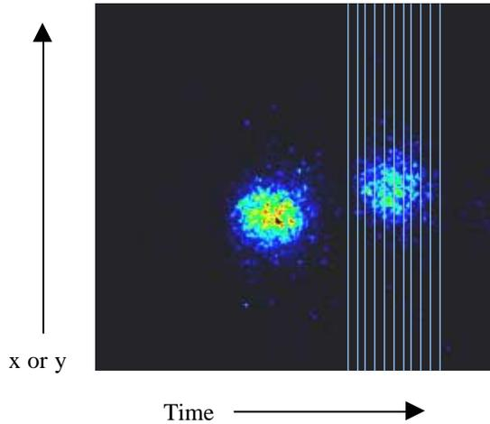
Figure 1: Typical streak camera data. The left streak image is  $y(t)$  and the right is  $x(t)$ . The lines on the image illustrate how the data-analysis software slices up the time-resolved image into 1-psec bins.
