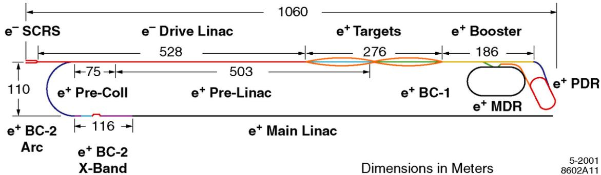
Figure 1: Layout of the NLC Positron Injector System for the cut-and-cover configuration (see section 2).
