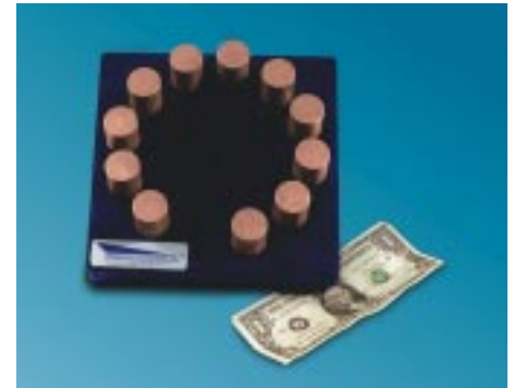
Figure 1: 9.0 kV, 30 A Solid-State Switch Module
