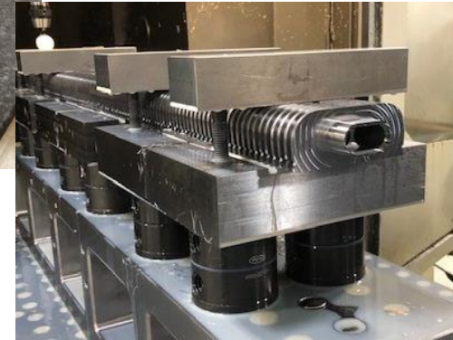
Single piece 1.1 m long magnet design
