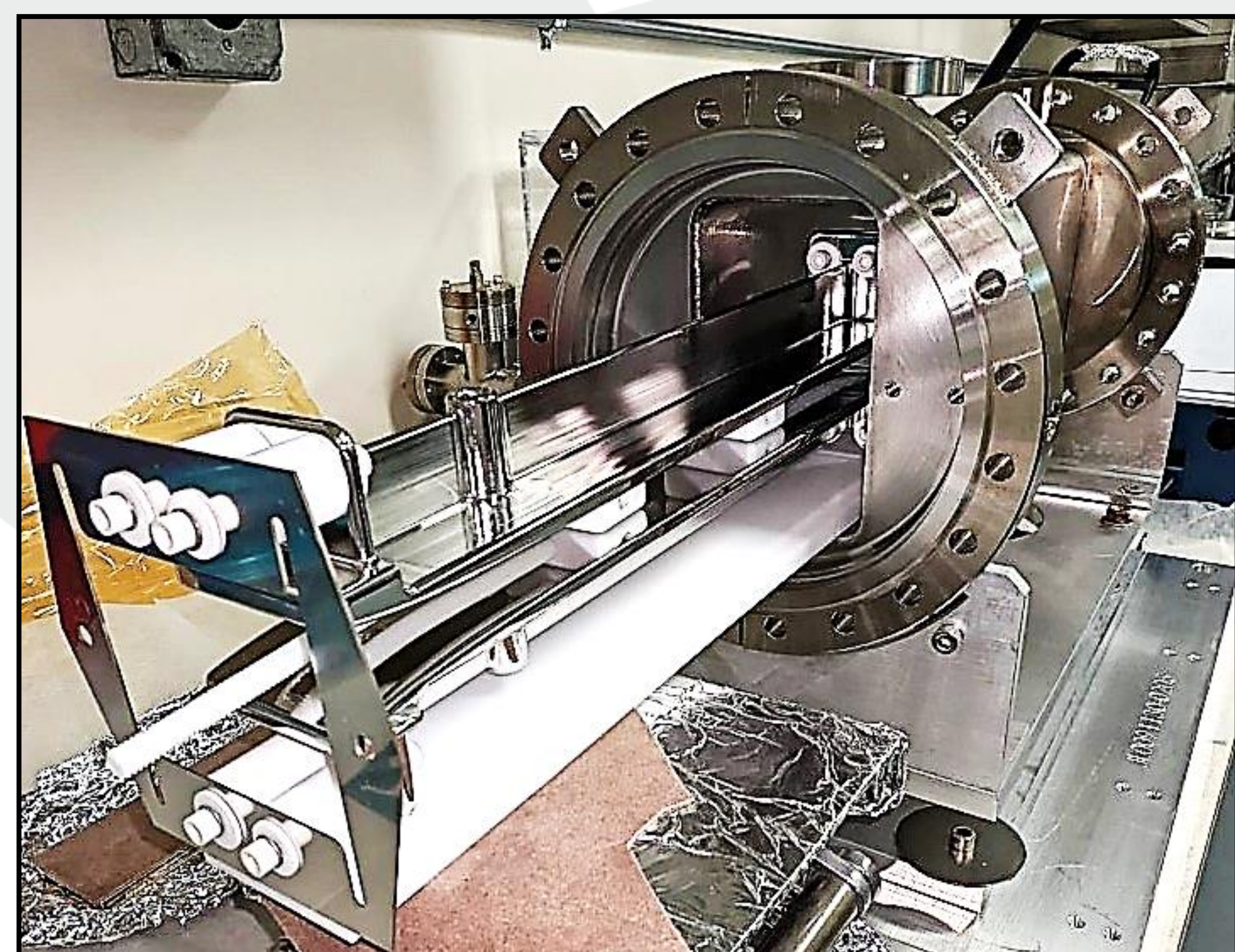
Picture of Wien filter during assembly.
