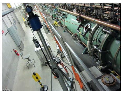
Setup for misalignment measurements in Drift Tube Linac
