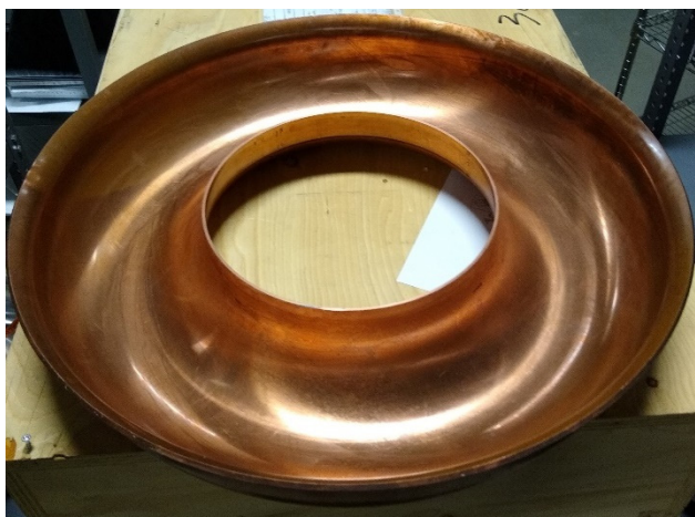
Figure 3: hydroformed copper test piece of the “short plate” (upstream end of the gun cavity). The outer diameter is approximately 0.6 m.
