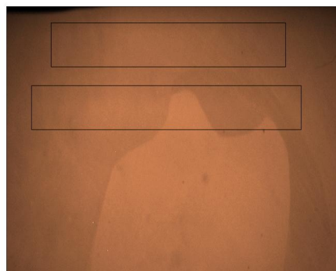
Figure 2: Fuzzy RHEED pattern observed from Cs 3 Sb cathodes grown on STO substrate via deposition-recrystallization method. The fuzzy features have been marked out using rectangular textboxes.
