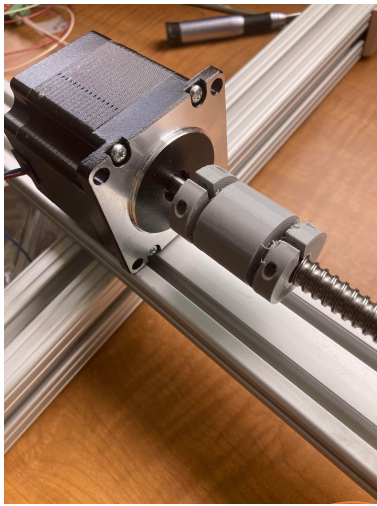
Figure 3: 3D printed coupler fitted to motor and ball screw. Slits on both sides of the coupler provide flexibility.
