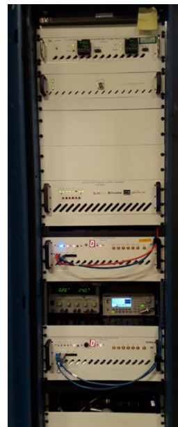
Figure 2: ACM test stand with one receiver, one tone generator, and one cavity (not visible).
