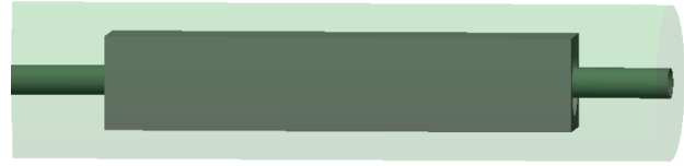
Figure 3: S-bend construction in BDSIM using the new feature. The outer geometry provided as one continuous piece by the user is implemented for the S-bend assembly. The magnet container logical volume is represented in light green.
