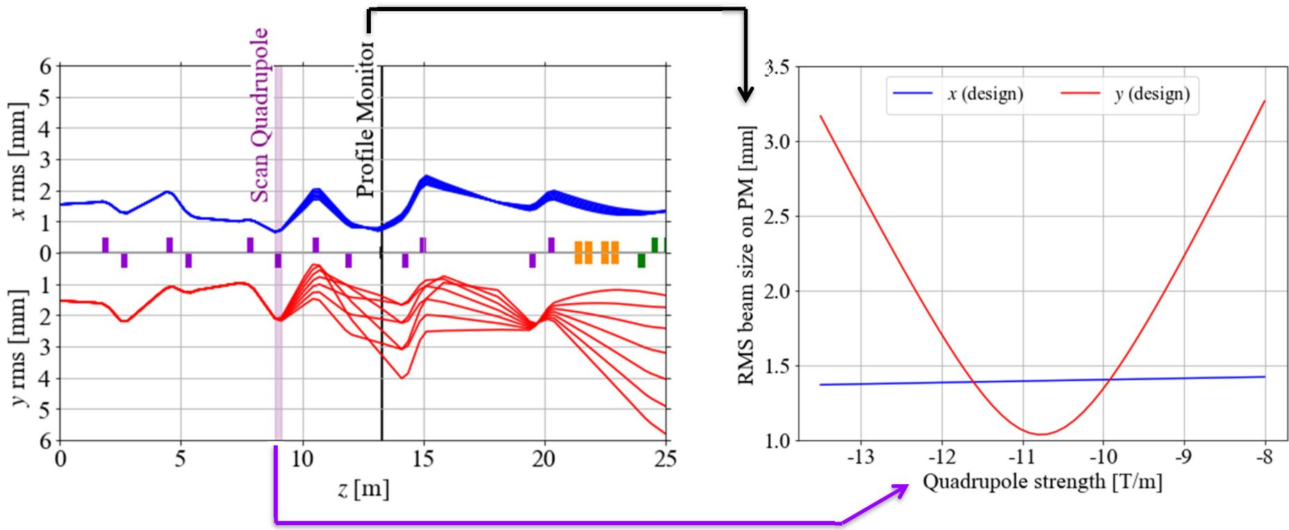
The above Q-scan setting is most suitable for the measurements in vertical ( $y$ ) plane. Similarly, the measurements can be performed in other phase space plane with high accuracy by scanning another quadrupole.
