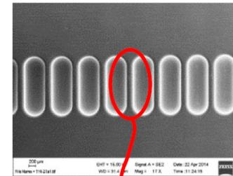
Cells 16-23, fist signs of damage
