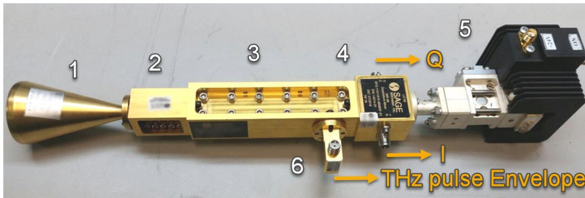
1 – 30-dB horn antenna, 2 – Band-pass filter, 3 – Directional coupler, 4 – IQ-mixer, 5 – Local oscillator, 6 – Schottky amplitude detector.
