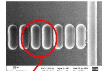
Output coupler, massive breakdown damage
