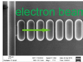
Input coupler, cells 1-7, no damage
