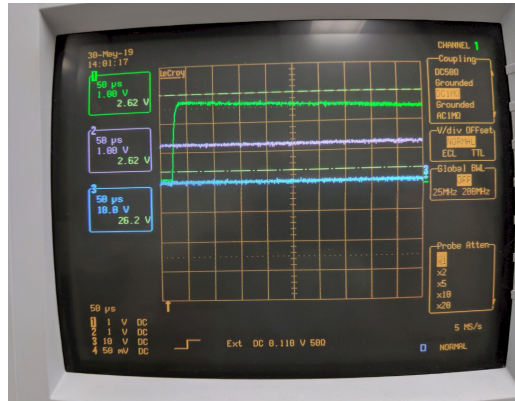
The signal is about 2.7V for 28nC
