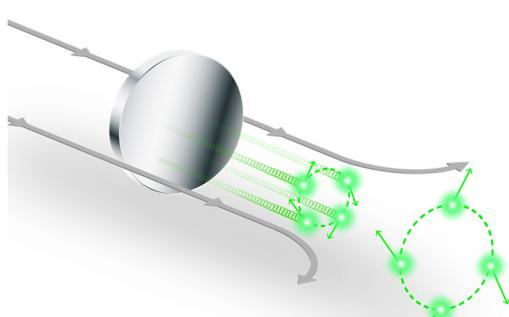
To implement cooling inside a solenoid, electron beam must be generated inside a magnetic field. Otherwise, electron beam will have mechanical angular momentum inside cooling solenoid per Busch's theorem, induced by radial fringe field as electron beam enters solenoid.
