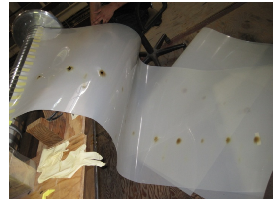
MYLAR Electrical Insulator damaged at flute location
