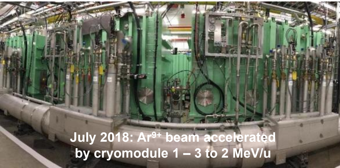
FRIB linac segment 1 containing 16 SRF cryomodules
