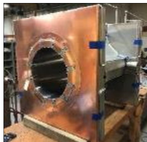
FSQ5 magnet thermal shield (South Holland, IL)
