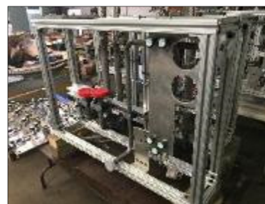
HWR cryomodule cryogenic manifold assemblies (South Holland, IL)
