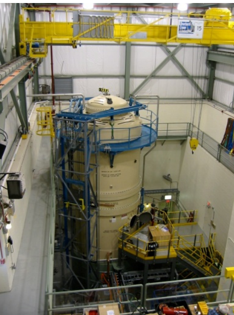
The Pelletron and beam “supply” and “transfer” lines
