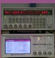
Figure 4: Top unit, Stanford Research Systems DG645 provides the trigger pulses to start and stop the drive signal. Bottom unit, FS740 with rubidium oscillator which disciplines the MO and DG645 via a 10 MHz reference. Long term timing is provided by the timing signals picked up from the GPS network.
