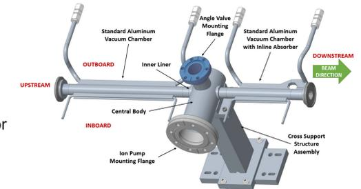
Typical NEG-coated aluminum vacuum chamber
