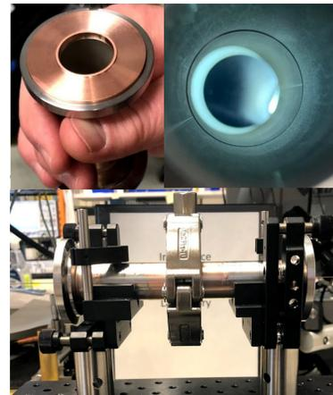
Custom RF sealing copper gaskets test on Goubau line and in-ring installations
