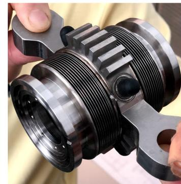
Recent prototype of APS-U beam position monitor with welded bellows
