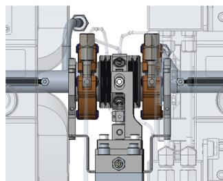
Beam position monitor (70 mm) & chamber supports
