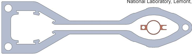
Existing 318 mm wide APS storage ring chamber compared to new APS-U chamber
