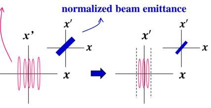
The normalized projected transverse emittance can be reduced with the collimator.
