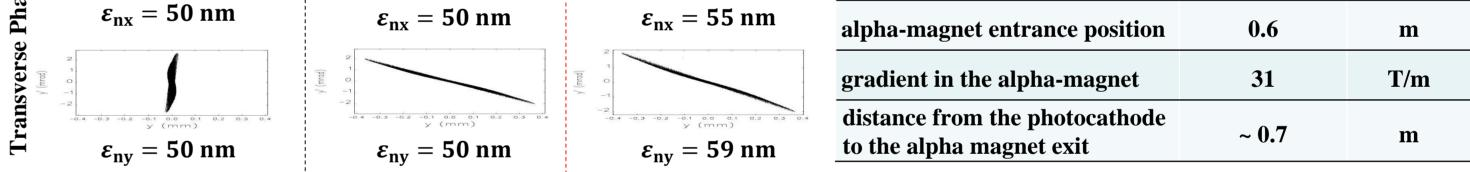
We have optimized the beam parameters at the exit of the alpha-magnet with energy slits as above. The alphamagnet was optimized to have the minimum bunch length at the exit of the magnet. When we compare the present simulation result with the design goal, the transverse beam parameters are not satisfied yet. Now, the optimization for the collimation and transverse beam emittance compensation are ongoing to meet the design goal.
